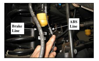
5. Carefully lower the rear axle enough to remove the coil springs from the rear spring pockets. Save the factory isolators for reinstallation.
