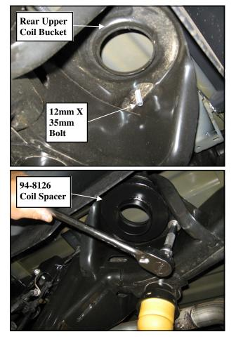
7. Reinstall the rear spring assembly into the rear axle spring perch. Make sure the pig-tail of the spring and **OE** isolator properly indexed in the mounting pocket.
