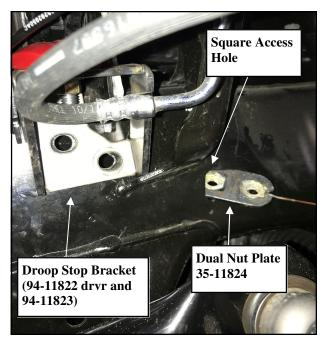
Install the droop stop bracket (94-11822 drvr and 94-11823 pass) to the frame and secure using the supplied 12mm X 30mm bolts and washers. Torque the 12mm bolts to 55 ft./lbs.
