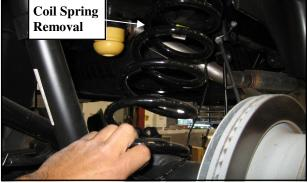
6. Install the rear coil spacer (94-11826) into the upper coil bucket by securing it with the supplied 12mm X 35mm bolt and hardware.
